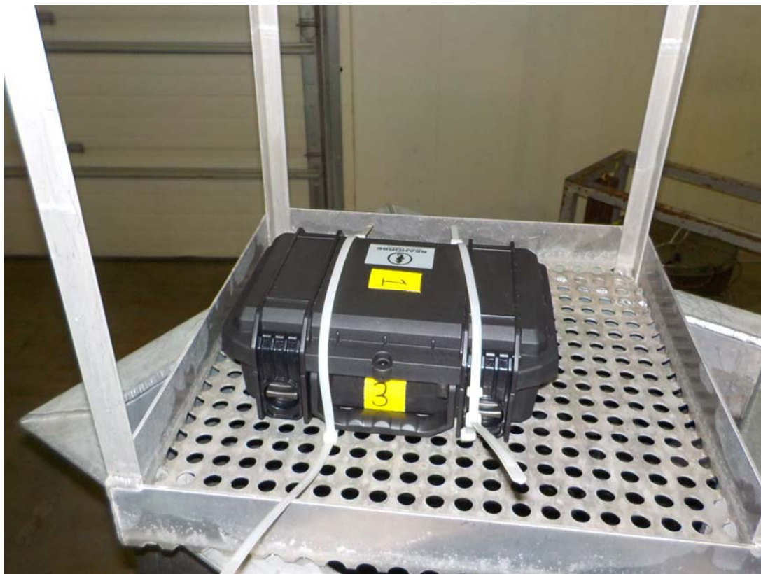
Photograph 4-2: Water Intrusion (Immersion) Test setup for test unit UUT-58687-2
