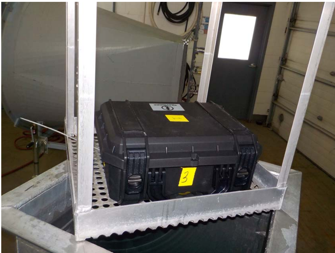
Photograph 4-4: Water Intrusion (Immersion) Test setup for test unit UUT-58687-3
